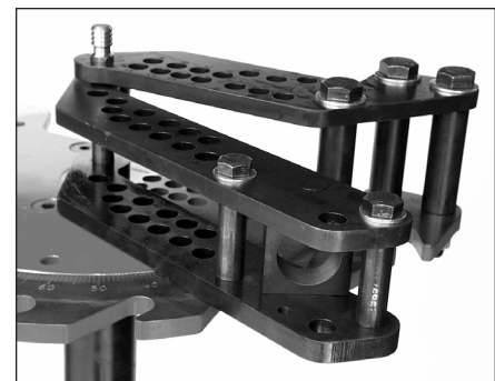
Figure 4 - Drive links installed
