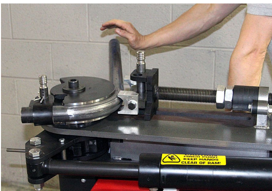
Striking the tube's end to loosen it from the pressure die
