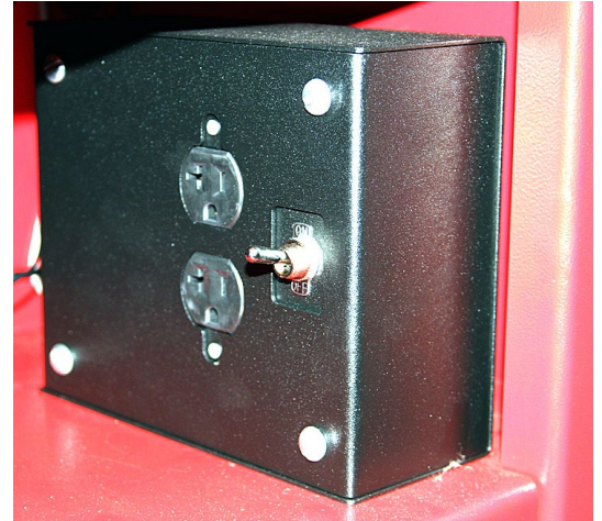
Auto stop control box installed in base
