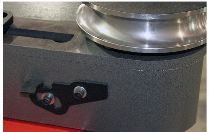
The spindle lock in the engaged DOWN position.
