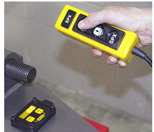
Computer at 0° ready to start bending
