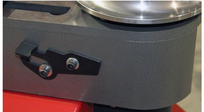
The spindle lock in the disengaged UP position.
