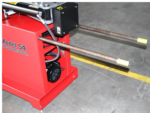
Bender shown with handles and the two rear leveling bolts installed.
