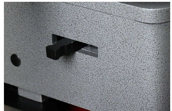
The spindle lock in the engaged position.
