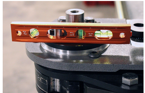
Spindle rotated in order to level front to back
