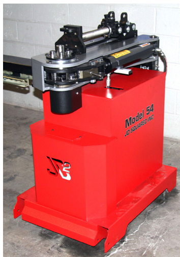
Bender mounted to floor
